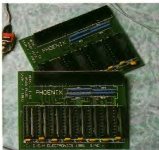
A500 Plus internal RAM expansions are becoming quite widespread - the Phoenix here is the first to arrive.
